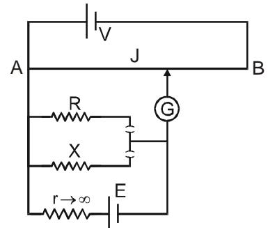
Here a battery with large internal resistance supply a constant current ( $i$ ) to either  $R$  or  $X$ . If it is connected to  $R = 10 \Omega$  potential drop across it will be  $iR$ , and the balance length is found to be 58.3 cm. If it is connected to  $X$  (unknown), Potential drop across it will be  $iX$  and the balance length is coming = 68.5 cm.
